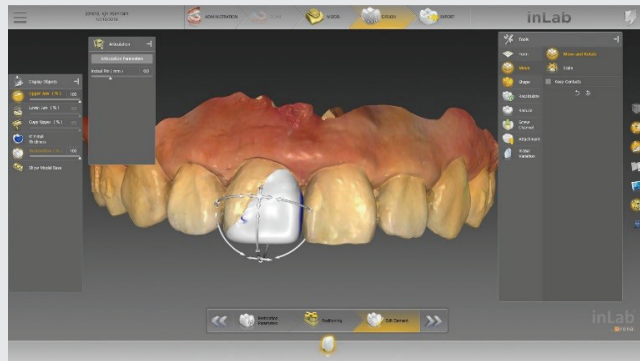
Figure 19. A partial veneer of the maxillary right central incisor was designed on CAD software (Inlab, Dentsply Sirona)
